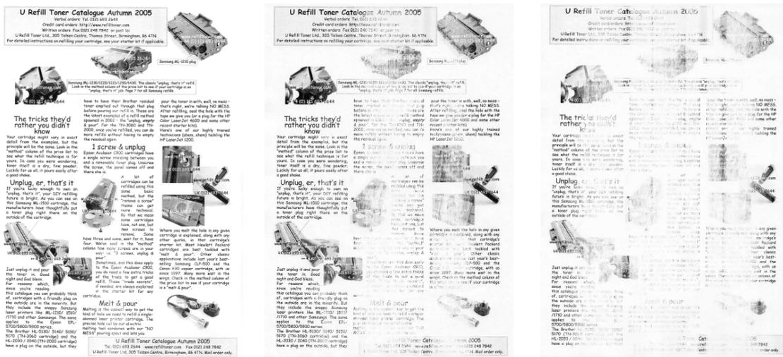
As you can see, the faded area gets wider and more pronounced with each print, but even on the last very faded page, the print at the edges is still the same blackness as on the first print. If you take out the cartridge and give it a shake at this point, perfect print will return for a few more prints – but then the fade out will return again. This pattern of progressively widening fade out bands which can be temporarily cured by shaking is the hallmark of toner exhaustion.
